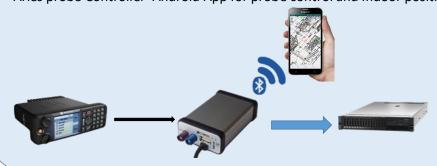
4) Voice Quality and SDS testing using a 2<sup>nd</sup> fixed transponder probe
