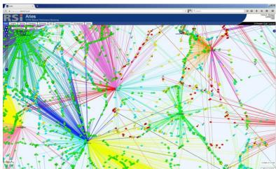
▲ Aries map showing the base site affiliation lines. The coverage areas of the sectored base sites can be clearly seen together with a small number of samples using what appear to be obviously wrong base sites – this is one of the ways that Aries helps to identify problems with handover and coverage leading to improved network performance for users.
